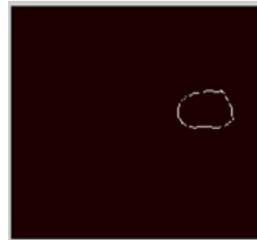
Fig.7: Tumor edge detection using 'Sobel' filter
