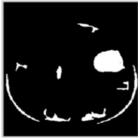
Fig.5: Objects left after filtering using area of binary objects
